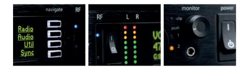
Left: Easily navigable grouped LCD menu Middle: RF mute switch and input level LED meter Right: Fast monitoring option for both channels including LED clip indicator
